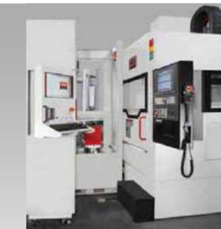
Manual operation position & Loading station
